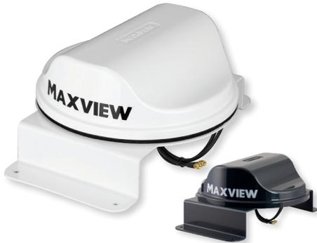
The raiser bracket allows you the flexibility to mount your antenna anywhere on your roof and enter the cable at your preferred point using the supplied cable entry cover. Alternatively you may have an existing cable entry point you may like to utilise instead.
